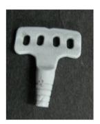
Fig. 6(a): Coated implant using EPD
